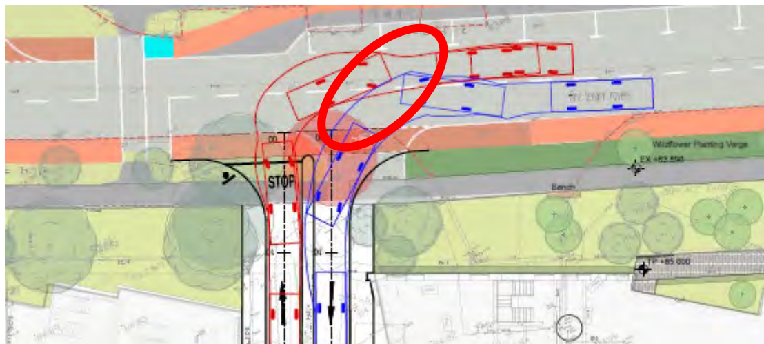
Figure 4 – Swept Path Analysis for Carmanhall Road Entrance
