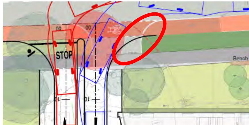
Figure 11 – Confusing kerb geometry alignment
